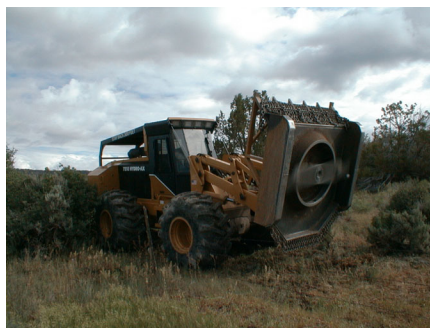
Figure 3. Mechanical treatment using a Hydroaxe®.
