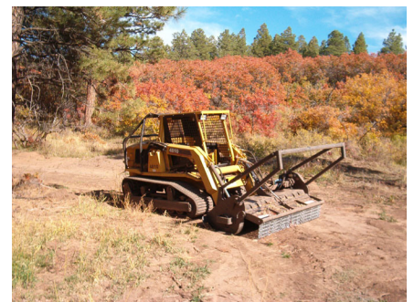
Figure 4. Mechanical treatment using a timberaxe.
